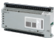
Micro U062: The low-cost telecontrol system for RTU stations with small data volumes, ready to connect
